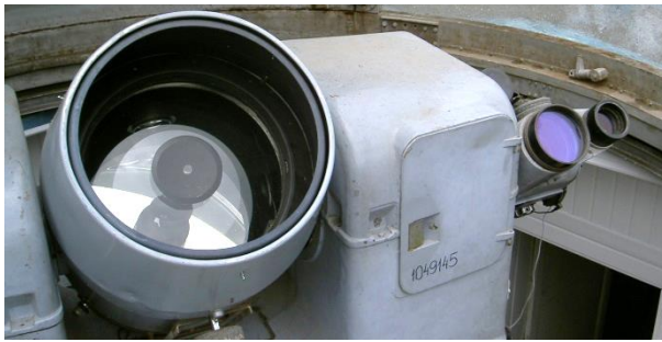
Figure 1: (Right) – Alt-azimuthal KT-50 telescope (photo); (Left) – Optical scheme of telescope.
