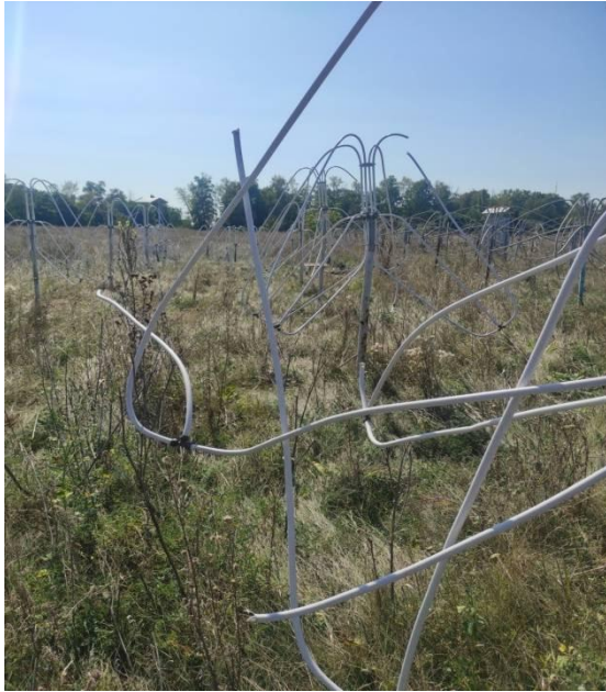
Figure 1: Damaged antenna elements of the GURT radio telescope.
