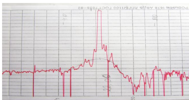
Figure 2: Sample 3C144 source record - April 22, 1988 (25MHz A -80m)
