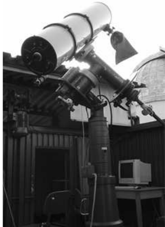
Figure 6: One of the small telescope, "Pupava" of 280 mm mirror diameter.
