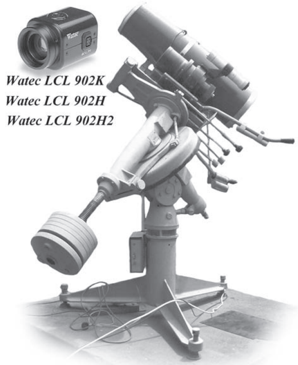
Figure 3. The meteor patrol on the base of the Schmidt telescope and the detector – WATEC camera
