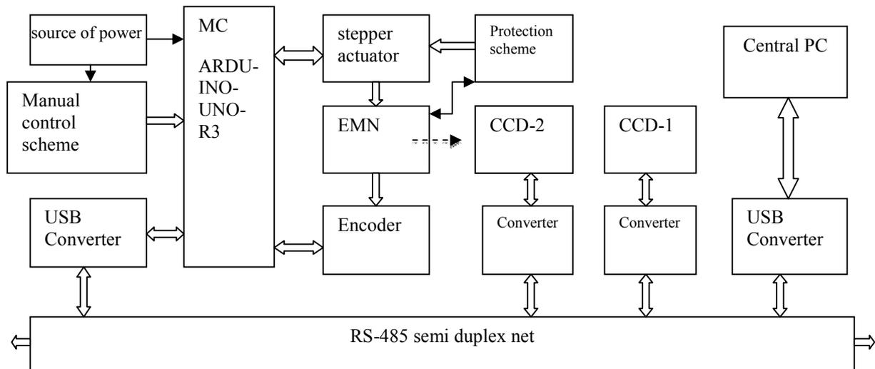
Figure 3: Structure of two-matrix photometer control system structure
