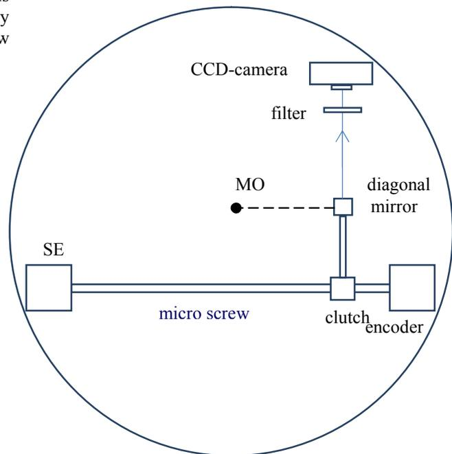
Figure 2: Optical-mechanical scheme of photometer second channel
