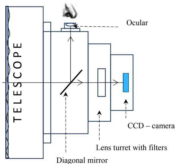
Figure 1: Optical scheme of photometer main channel
