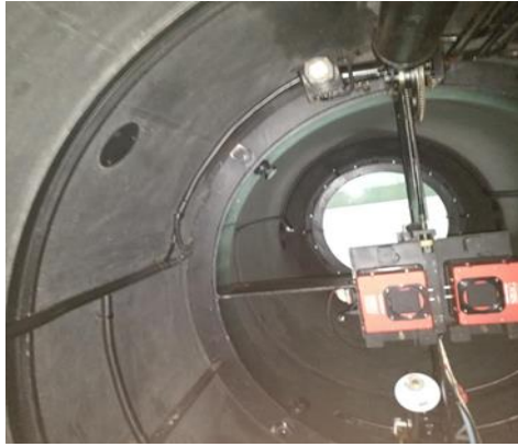
Figure 4: Two CCD cameras are located in the focal plane of the Schmidt telescope.
